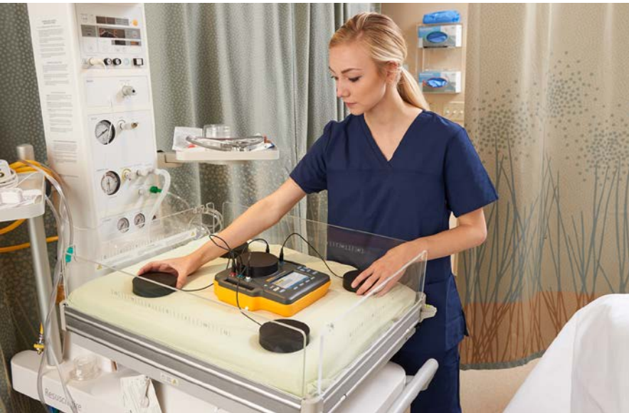
Pucks are used with the INCU II Incubator/Radiant Warmer to verify the performance of a radiant warmer
