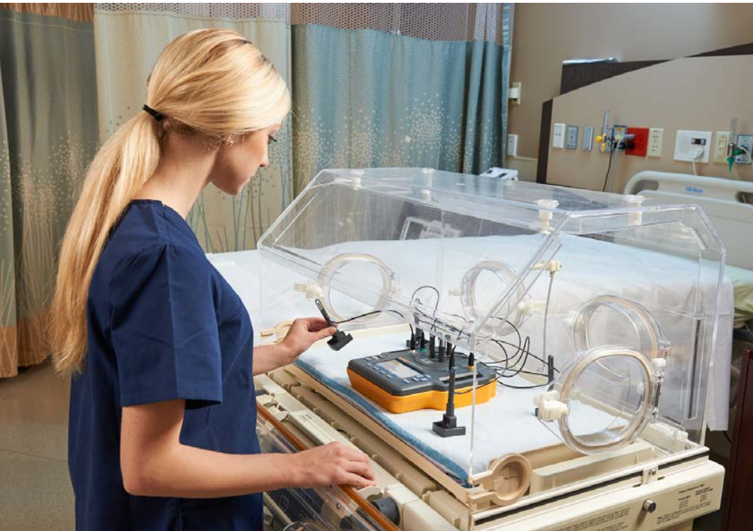
INCU II Incubator/Radiant Warmer Analyzer being used to test an infant incubator
