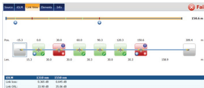
Figure 4: Measurement of fiber 3 using an iOLM-OTDR, after correct mating of connector 2.
