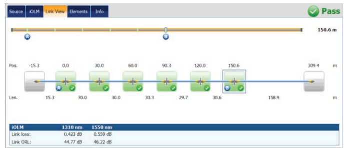
Figure 8. Measurement of fiber 3 using an iOLM-OTDR, after repairing the macrobend at connector 6.
