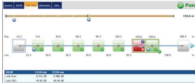
Figure 7. Measurement of fiber 3 using an iOLM-OTDR, after cleaning connectors 2 and 6.
