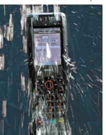
and water according to the IP67 protection class and is fully functional at temperatures between -20°C and +50°C. Come rain or shine - or even at extremely cold temperatures - the CASIO DT-X200 has the ideal features to prove its worth in the long-term when used in tough working conditions. The balanced design and the non-slip surface on the bottom of the device allow it to be operated easily and effortlessly.
