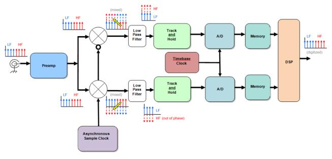
Figure 12. ATI Channel Block Diagram.
