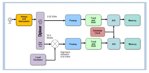
Figure 5. Example of a mixer-based acquisition channel.
