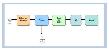
Figure 1. Conventional Analog-to-Digital acquisition channel.
