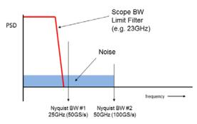
Figure 4. Nyquist bandwidth extension as a result of time interleaving.
