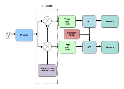
Figure 10. Asynchronous time interleave circuit.
