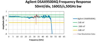
Figure 7. Agilent DSAX95004Q frequency response plot.
