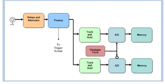
Figure 3. Time interleaved A/D converters.
