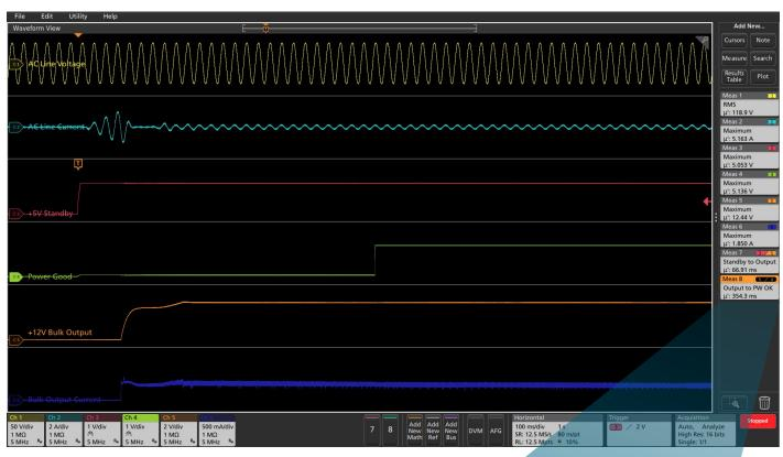
AC/DC switching power supply turn-on after front-panel switch was pressed
