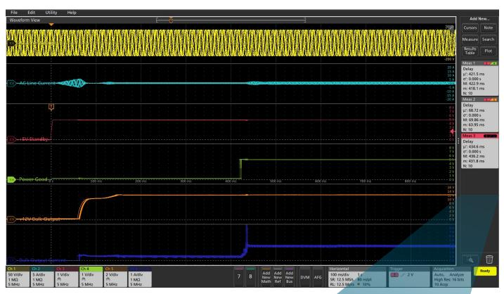
Repetitive turn-on timing measurements with infinite persistence and measurement statistics
