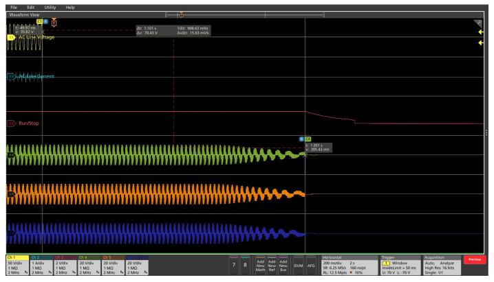
3-phase motor drive turn-off delay measurement after AC mains was disconnected
