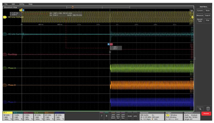
3-phase motor drive turn-on delay measurement after AC mains was connected
