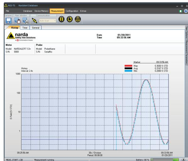
Fig. 6. Real-time measurement display of exposure over time
