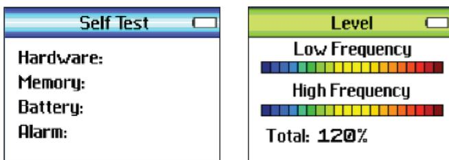
Fig. 2. Self-test screen and normal operation display
