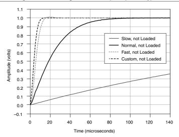
Figure 3. 1 mA Range No Load Step Response, Typical
