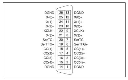
Figure 3-2. NI 1433 Base Configuration MDR Connector Pin Assignments
