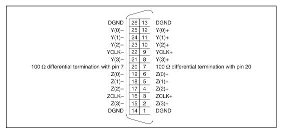
Figure 3-3. NI 1433 Medium/Full Configuration MDR Connector Pin Assignments
