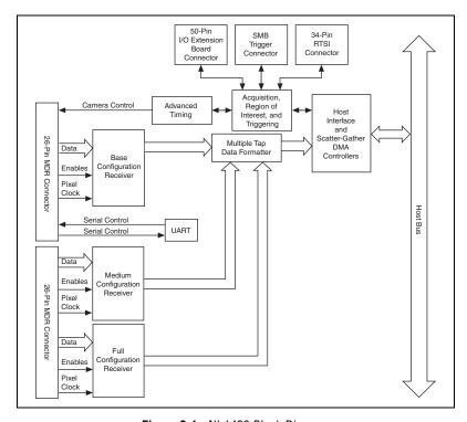
Figure 2-1. NI 1433 Block Diagram
