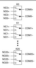
Figure 2. NI PXI-2523 Connector Pinout
