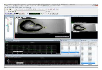
TEMA is used to calculate the rotational volume of the cavity created by the bullet fired into the gelatine. Other parameters such as speed, acceleration, bullet orientation are also analysed.
