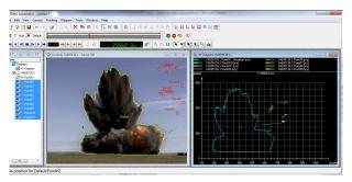
Single shrapnels are tracked as well as the actual explosion dynamics. Using withnessplates around the area will effectively give information about shrapnel size, speed and density.
