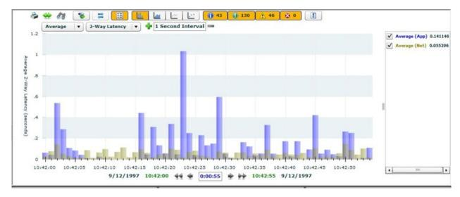
Ideally, network latency and application latency measurements can be graphed together over time. Comparing the measurements and seeing the differences can provide information that might have otherwise been overlooked, and aid in identifying transient application problems.
