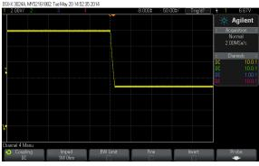
PS48402 step response (12V-5V step programmed,  $82\Omega$  load)
