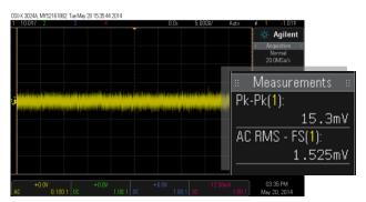
PS48402 output noise (20Hz-1MHz BW, 24V, 82Ω load)
