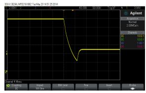
Competitor step response (12V-5V step programmed,  $82\Omega$  load)
