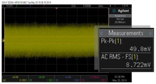
Competitor output noise (20Hz-1MHz BW, 24V, 82  $\Omega$  load)
