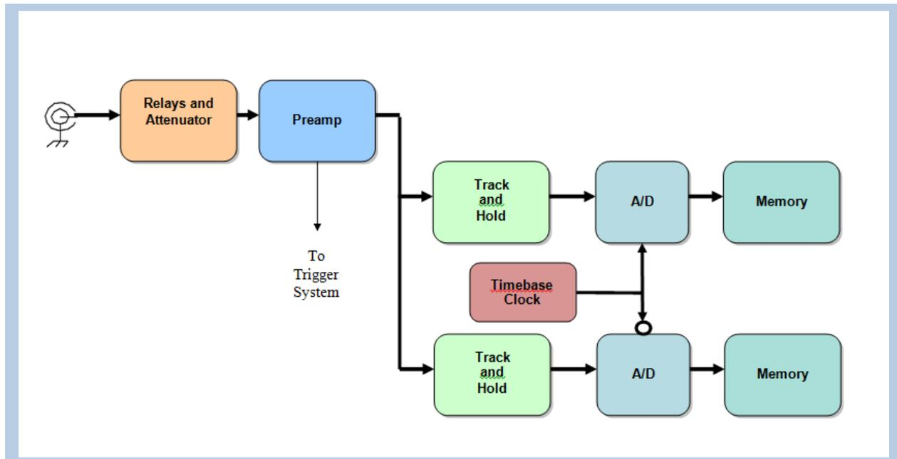
Figure 3. Time interleaved A/D converters.
