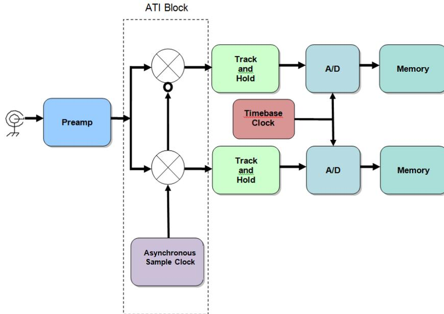
Figure 10. Asynchronous time interleave circuit.
