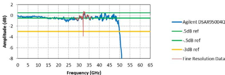
Figure 7. Agilent DSAX95004Q frequency response plot.
