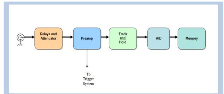
Figure 1. Conventional Analog-to-Digital acquisition channel.
