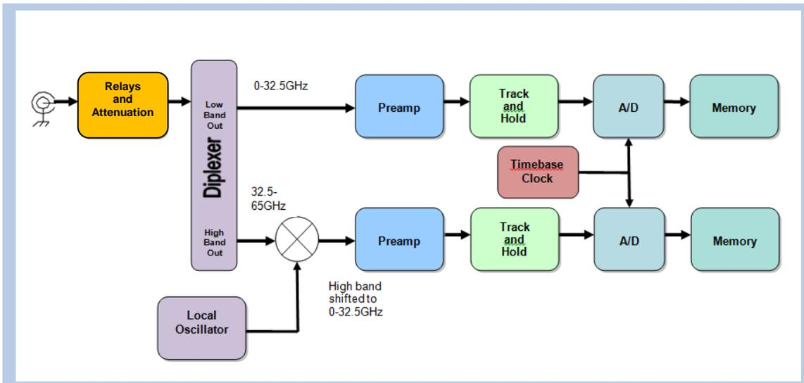
Figure 5. Example of a mixer-based acquisition channel.
