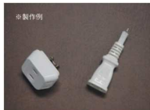
Connection jig Made it accordance to the DUT with safety in mind
