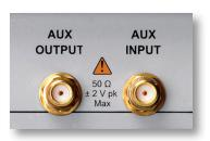
These can be used to test the instrument's inputs, experiment with its features and verify complex setups such as mask tests. AUX OUTPUT can also be configured as a trigger output.
