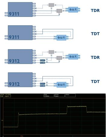
The PicoScope 9312 is supplied with the 9040 and 9041 external tunnel diode pulse heads that generate positive and negative 200 mV steps with 40 ps rise time. The PicoScope 9311 generates large-amplitude (6 V) differential 60 ps steps with 65 ps rise time directly from its front panel and is suited to TDR/TDT applications where the reflected or transmitted signal is small.
