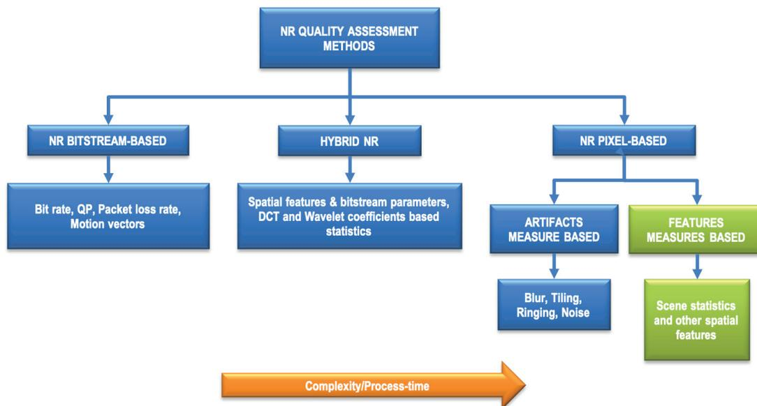
Figure 7. Hierarchy of NR methods vs. complexity and performance.
