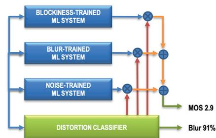
Figure 4. TekMOS ML algorithm feature vector combined into regression and classification results for pooling MOS scores and dominant distortion class.
