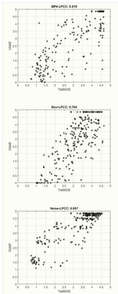
Figure 6. Netflix's full-reference VMAF scores Vs TekMOS' s no-reference scores.
