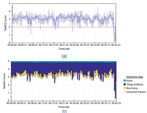
Figure 2. Example graph from file-based video quality assessment. (a) TekMOS scores for entire video stream shown in one graph and, (b) shows the probability that the resulting score is caused by one of the distortion classes.
