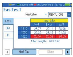
Within 10 seconds, the MaxTester's FasTesT function provides insertion loss and ORL values for up to three wavelengths—including either 1490 or 1625 nm—on a single port.
