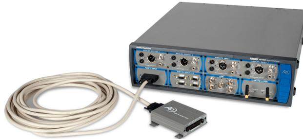
APx525 with PDM 16 module attached to remote interface pod
