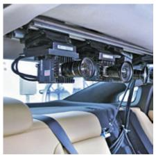
Phantom Miro C320J cameras installed on-board for a crash test
