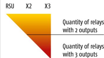
RSU 2223 = 2 relays with 2 outputs and 2 relays with 3 outputs
