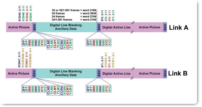
Figure 17. 2048x1080 R'G'B' 12-bit Dual Link data structure format.
