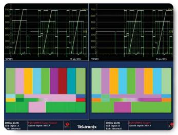
► Figure 3. Waveform displays of Dual Link A and B signal for R'G'B' (A) 4:4:4:4 format.
