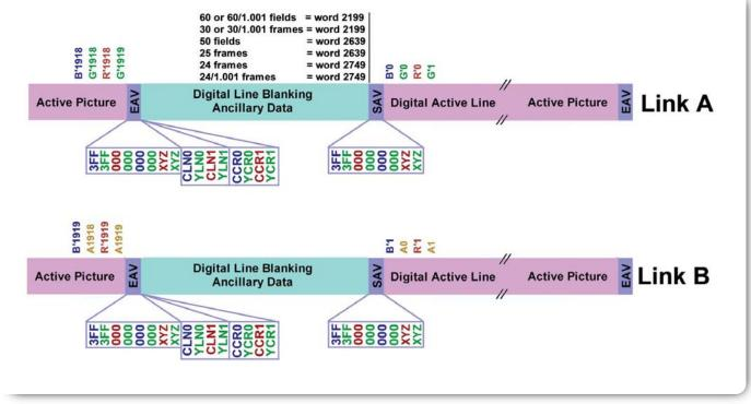
▶ Figure 6. Data Structure of R'G'B'(A) 4:4:4:4 format for both Link A and Link B.
