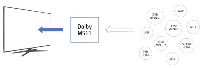
MS11-compliant products can accept Dolby Digital Plus™, Dolby Digital, Dolby Pulse, and other AAC bitstreams as input. MS11 decodes the input bitstreams to produce PCM output and also transcodes or converts the input from its original format to the Dolby Digital format to support existing products that only contain the Dolby Digital decoders. The MS11 Decoder can pass through an encoded audio stream for decoding in other products, such as an audio/video receiver (AVR).
