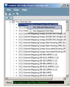
To run an entire test sequence, click the *Start Sequence* button ( symbol) located just above the navigator tree. To run a single section, such as "Two Channel Line," right click on the section name and choose *Run Selected Signal Path* in the navigator tree (see above middle). To run an individual measurement, right click on the measurement and
