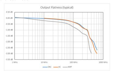
AMP (1  $V_{p\text{-}p}$  Sine wave, relative 1  $\mu\text{Hz}$  to  $\leq$  10 MHz:  $<\pm0.5$  dBc to 1 kHz)
