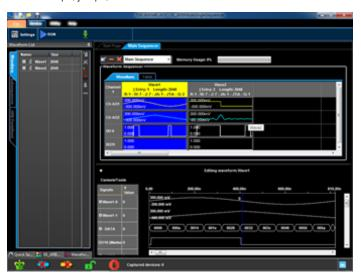
In the Multi-sequence mode, two sequences can be defined to control Channel 1 and Channel 2 (and the corresponding digital channels) separately as two units of generator.
