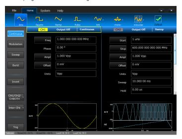
In Advanced mode, users can define complex waveforms with up to 16,384 entries of analog waveforms and digital patterns in a sequence, in terms of loops, jumps, and conditional branches.
