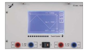
The freely programmable mode makes it possible to program up to 6 curves each with 99 support points. In this mode, one always presets the start value and end value for current and voltage, and also the duration. In the automatic and rotary switch versions, the arbitrary function can be used only via the interface.
