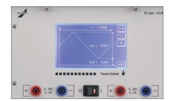
The freely programmable mode makes it possible to program up to 6 curves each with 99 support points.
