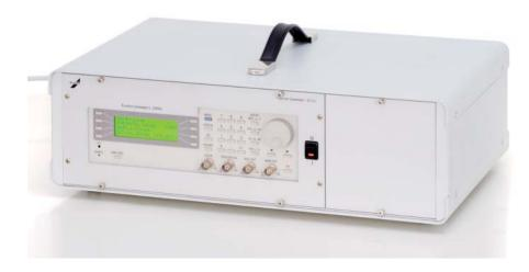
The aluminum shell housing enables the mobile utilisation of Elabo 3HU eurocassettes. Aluminum traverse profiles are mounted inside with M 2.5 threads at the front and the rear in 5.08mm separation grids in accordance with DIN 41494. A female multipoint connector with 11 high-current contacts serves as the insert mating connector.
