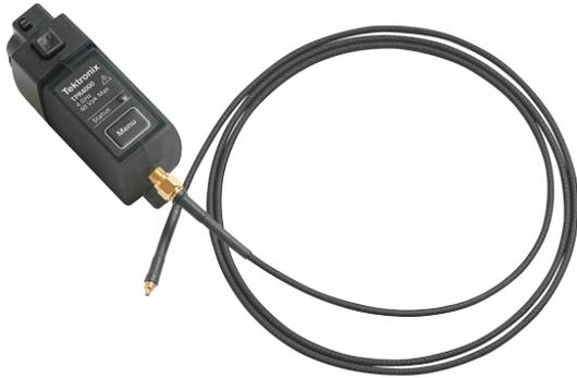
The TPR1000 and TPR4000 probes provide a low noise, large offset range solution for measurement of ripple on DC power rails ranging from –60 to +60 VDC. Tektronix’s power rail probes offer industry leading low noise and high offset range required to measure AC ripple between 200  $\mu\text{V}_{\text{p-p}}$  and 800  $\text{mV}_{\text{p-p}}$  at up to 4 GHz.
