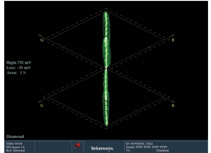
Figure 22. This is a Diamond display with a balanced chip chart.
