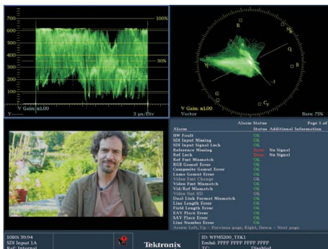
Figure 4. The Tektronix Waveform Monitor shows that the image doesn't take advantage of the full dynamic range. Blacks are lifted (above 0) and whites aren't at 100% (or 700 mv).
