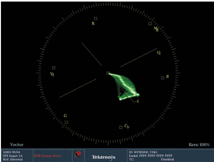
Figure 17. This Vectorscope is of a misbalanced Chip Chart. Because the Chip Chart is only made up of black, white and gray chips, the entire trace should be very close to the center. This image shows the trace skewed far off towards the blue vector, indicating a very blue image.
