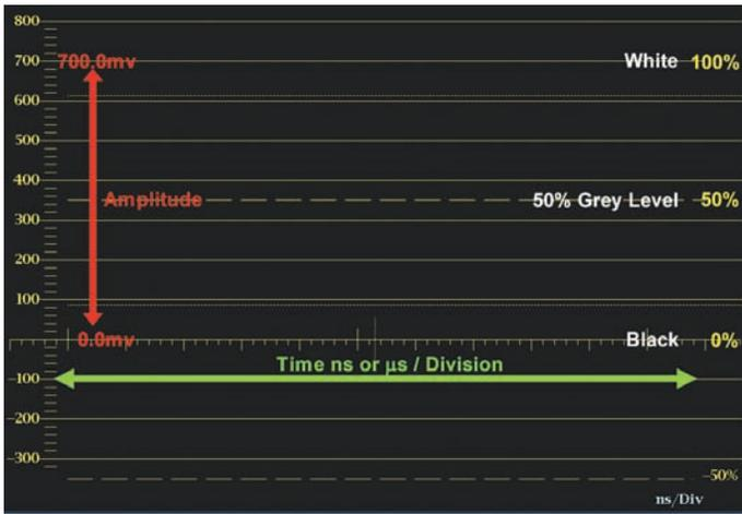
Figure 1a. Waveform display.
