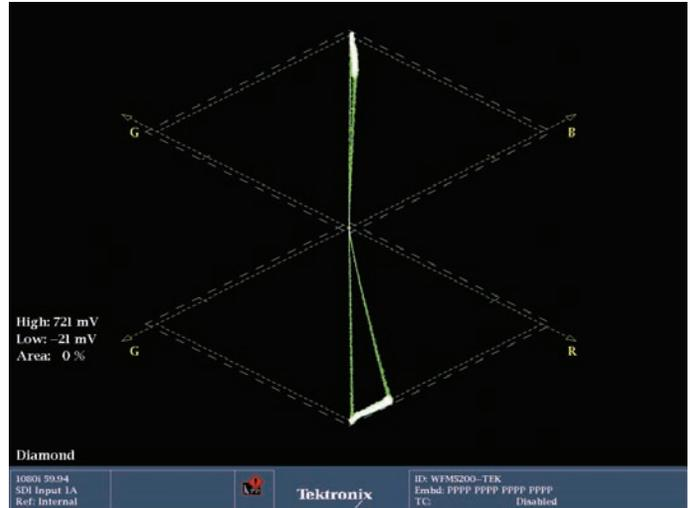
Figure 7. Diamond display with Red gain in balance.
