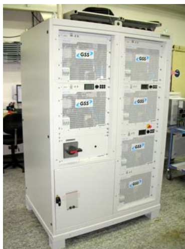
Picture 2: 192 kW battery simulator, nominal output voltage up to 1500 VDC, depending on user defined master-slave configuration of the single devices. System contains 6 bidirectional DC power supply units TC.GSS.
