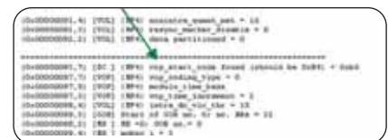
► Figure 8. Example of a Trace/Interpret output, at the start of an MPEG-4 VOP.
